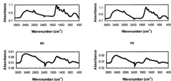
Figure 2. FTIR spectra for whole fish skin and commercial gelatin. SDC: Skin dried in silica gel at room temperature, SDO: Skin dried in oven at 80°C, BG: Bovine gelatin, PG: Porcine gelatin
