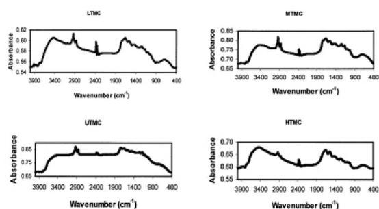
**Figure 4.** FTIR spectra of fish skin gelatin extract using 0.1 N acetic acid solution at different temperature. LTMC: 4°C and 0.1 N, MTMC: 20°C and 0.1 N, UTMC: 50°C and 0.1 N, HTMC: 80°C and 0.1 N
